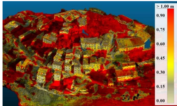
Fig. 5 Cloud-to-mesh comparison: computed distances (Croce et al., 2019).
