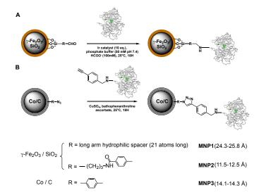
Scheme 2: Grafted core-shell MNPs. A: reductive alkylation; iron-oxide core/silica shell aldehyde particles; MNP1 = long arm hydrophilic spacer, MNP2 = aromatic spacer. B: azide-alkyne cycloaddition; cobalt core/carbon layers shell azido particles (MNP3); alkyne activated laccase (reductive alkylation). Approximative lengths of linkers (enzyme-to-shell) are given in brackets.
