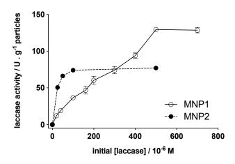
**Figure 2:** Initial laccase concentration *versus* immobilised laccase activity. MNP1 and MNP2 particles concentration 2 g.L<sup>-1</sup> incubated at 30°C in 0.1 M acetate buffer pH 5.5 in the presence of ABTS (5 10<sup>-3</sup> M final). Kinetics of the radical cation formation followed spectrophotometrically at 420 nm ( $\epsilon$ = 36 000 mol<sup>-1</sup> cm<sup>-1</sup>) for 2 min.
