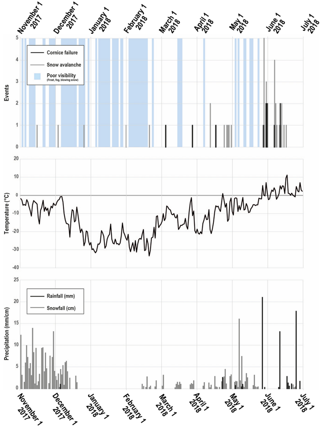
Fig. 5. Occurrence of cornice failures and snow avalanches during the winter/spring of 2017–2018, as observed on TAS1 and TAS2 cameras. Maximum air temperature and precipitation are also shown (source: CEN 2018 , Environment Canada 2021 ).
