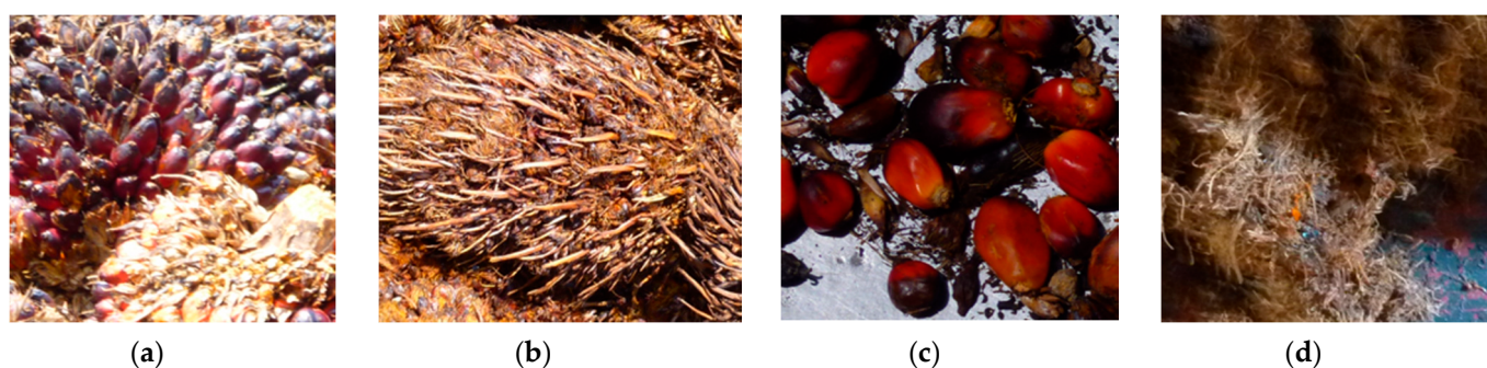
Figure 2. POFL bundle with fruits and after grinning ((a,b) respectively), palm oil fruit and POFR short fibers ((c,d) respectively).
