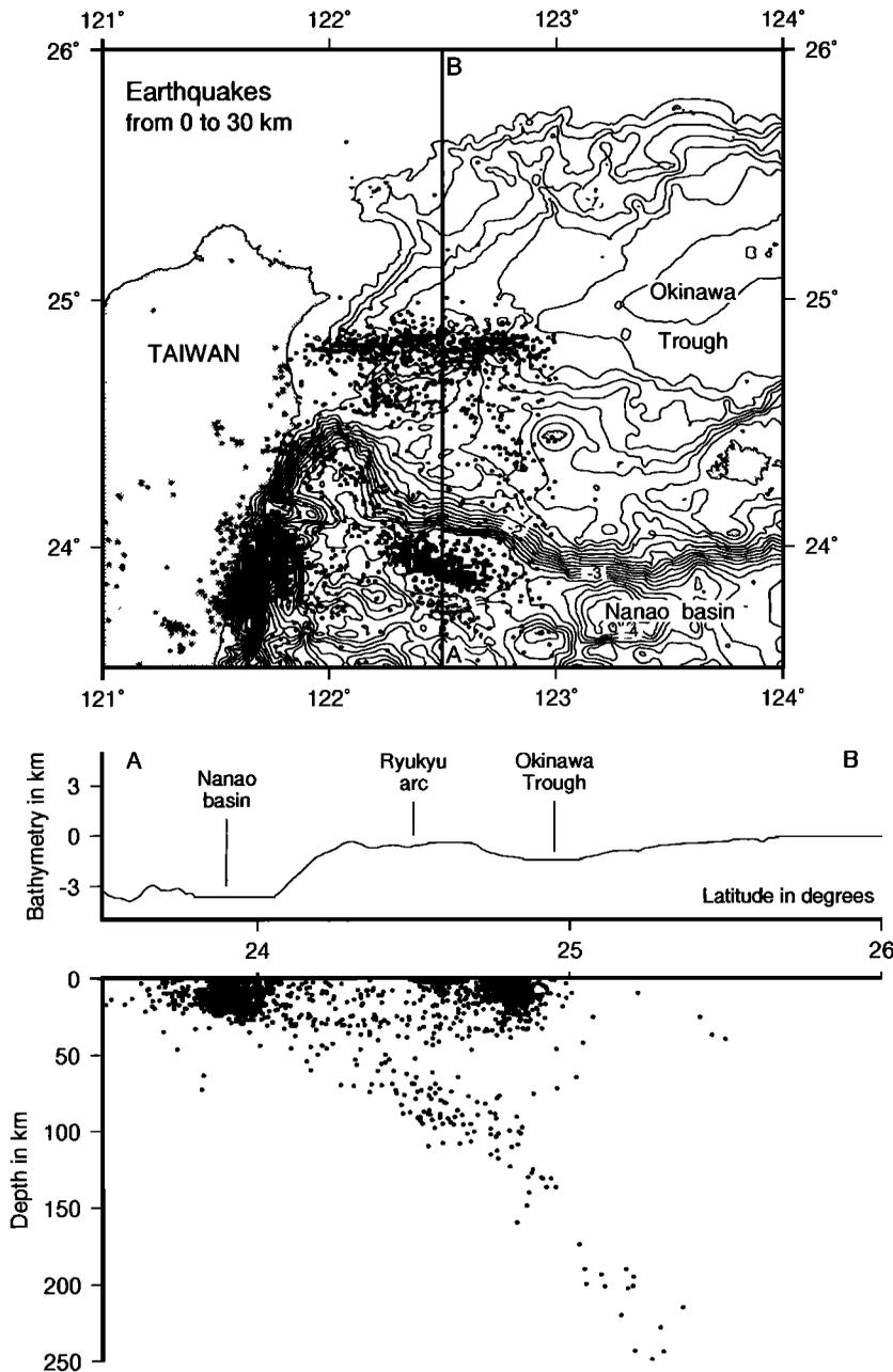
**Figure 8.** (top) Location of 0- to 30-km-deep earthquakes west of 123°W longitude (Telemetered Seismograph Network (S.-N. Chen, personal communication, 1996)) on the bathymetric map contoured every 250 m. (middle) and (bottom) N-S cross-section at 122°30'W (AB). Crustal earthquakes are mostly located on the southern margin of the Okinawa Trough where small offset normal faults are observed (Figure 9).
