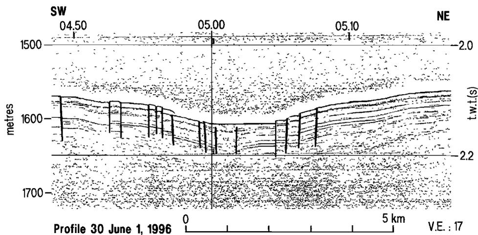
**Figure 9.** Portion of the 3.5 kHz profile 30 (location in Figure 2) located across the seismic area with the presence of a slight depression (also displayed on the seismic profile 30, Figure 6). Normal faults with a mean spacing of about 600 m present offsets of a few meters.
