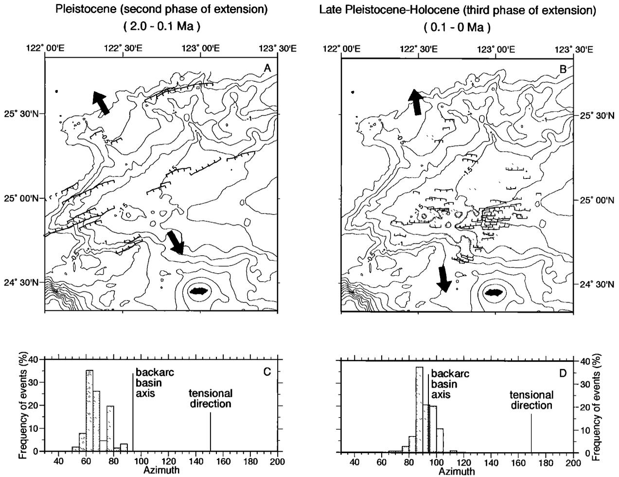
**Figure 11.** (top) Distributions of the two simplified normal faults systems associated with the two last phases of extension in the southwestern Okinawa Trough as well as the inferred direction of extension (large arrows). (bottom) Frequency of normal faults segments in function of their azimuths and deduced tensional directions from comparison with analog modeling results.
