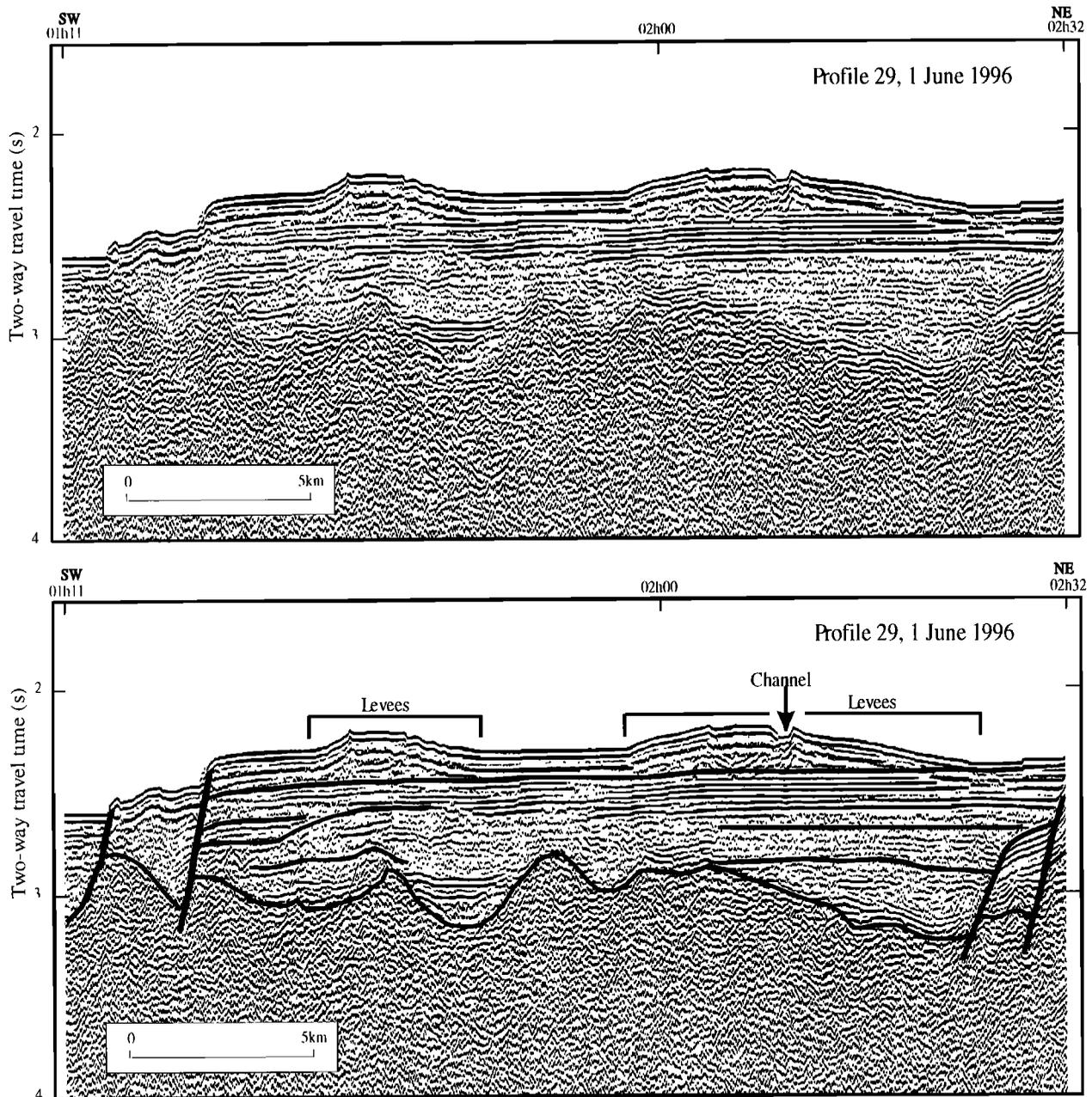
**Figure 10.** Migrated six-channel high-speed seismic profile 29 (location in Figure 2) across the extinct channel meanders located north of the backarc depression. Due to meandering, the seismic profile twice crosses the same submarine channel (Figure 2 and Plate 1). Note the presence of sedimentary levees about 150 m thick above the Pleistocene horizontal sedimentary sequence.
