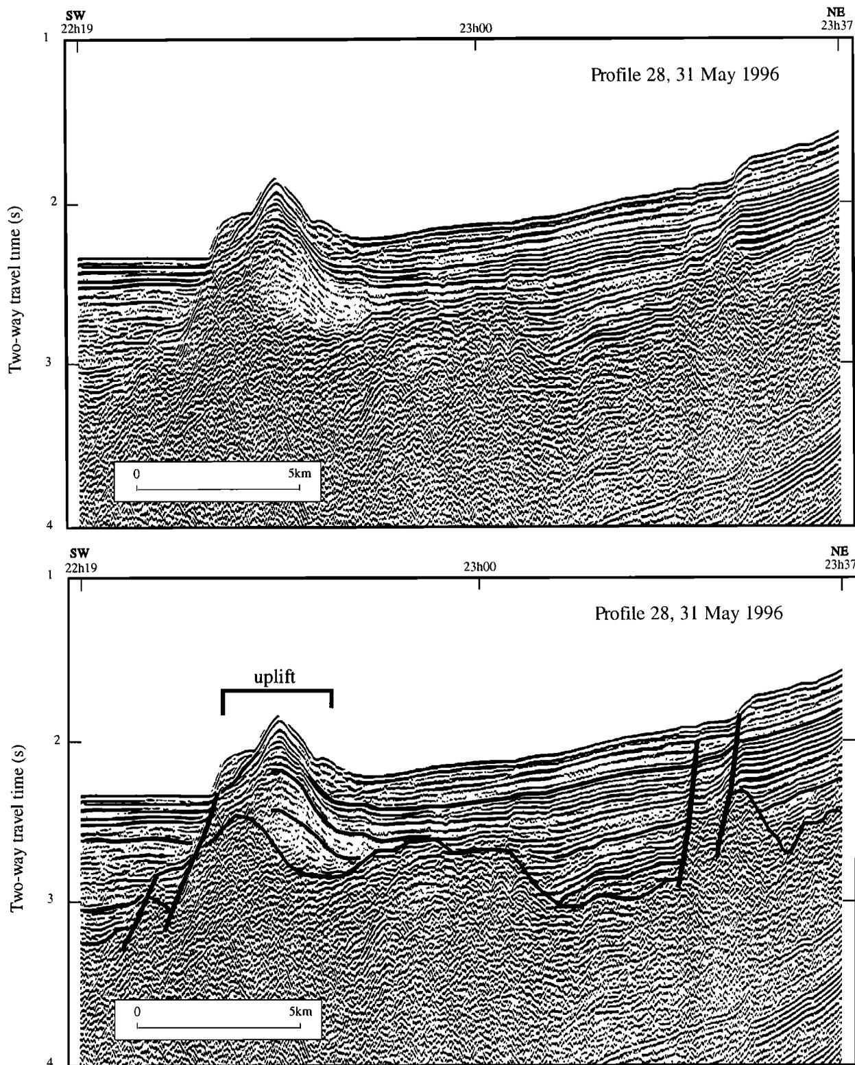
**Figure 5.** Migrated six-channel high-speed seismic profile 28 (location in Figure 2) across a major volcanic feature capped by undeformed uplifted sediments and bounded to the north by an ENE-WSW trend located at the base of the northern slope of the Okinawa Trough and to the south by a E-W normal fault (Figure 3).
