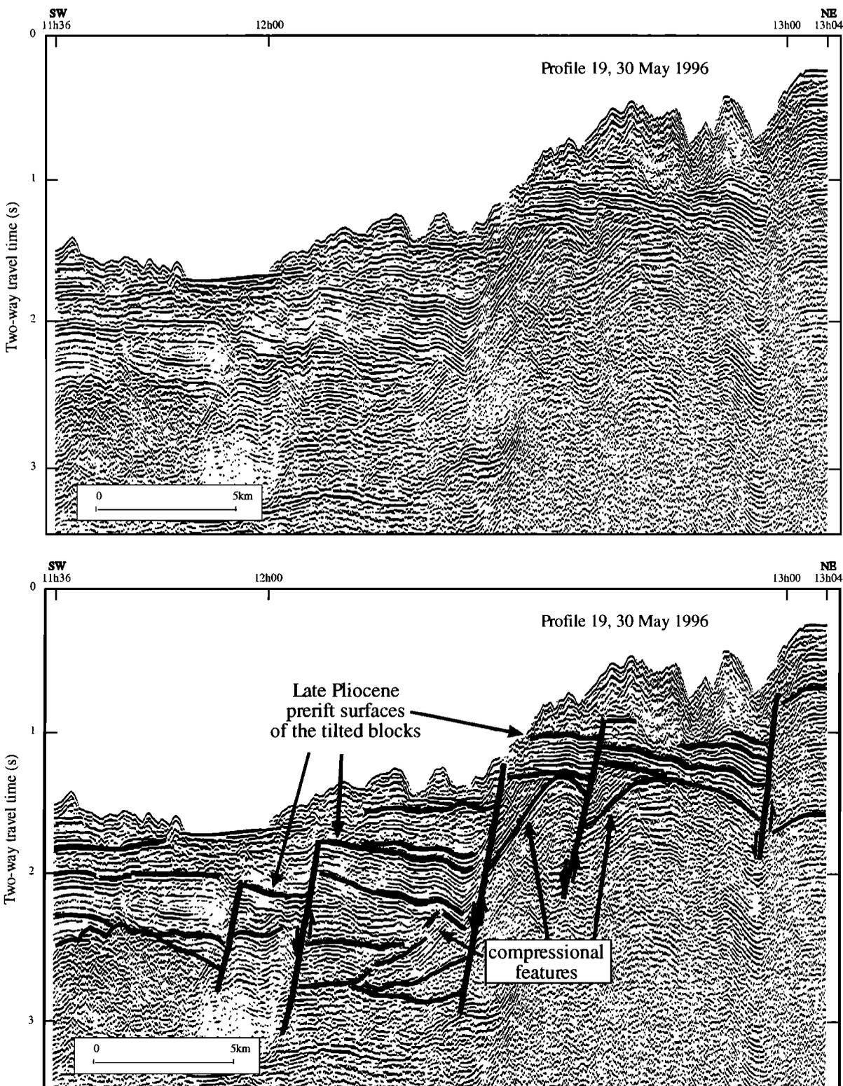
**Figure 4.** Migrated six-channel high-speed seismic profile 19 (location in Figure 2) across the northern OT margin. Example of tilted fault blocks formed at the Plio-Pleistocene boundary but showing internal deformations linked to late Miocene (6-7 Ma) tectonic compressive motions.
