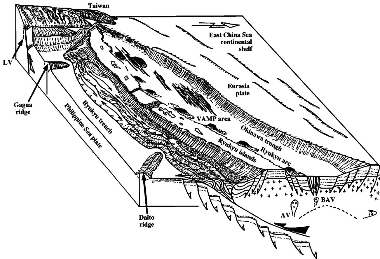
**Figure 16.** Three-dimensional artist view (B. Deffontaines) of the Ryukyu subduction system looking southwest with the three different types of volcanism (arc, backarc, and cross-backarc volcanisms) which appear in the Okinawa Trough. BAV, backarc volcanism; AV, arc volcanism; LV, Longitudinal Valley.
