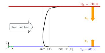
FIG. 1. Geometry of the channel flow. The periodic directions are in green.
