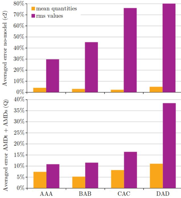
FIG. 7. Averaged errors obtained with four different meshes on mean quantities and RMS values. Simulations without model and with the tensorial AMD model are investigated.
