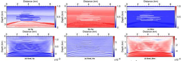
Figure 4: P-wave velocity (left column), density (middle column) and  $Q^{-1}$  (right column): normalized models (first row) and preconditioned gradients of the 1st iteration (second row).
