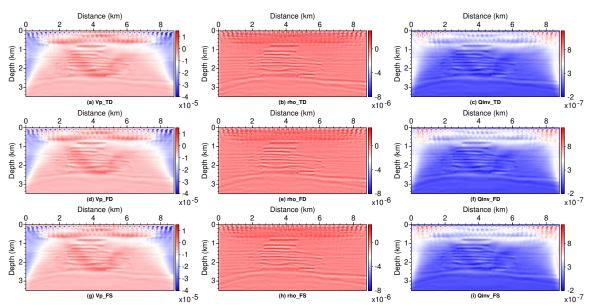
Figure 8: FN Hessian-vector product: P-wave velocity (left column), density (middle column) and  $Q^{-1}$  (right column). Time-domain implementation (first row), frequency-domain approximation (second row) and full-scattered-field approach in frequency domain (third row). 25 frequencies are used in two approximate methods.
