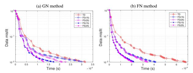
Figure 11: Comparison of convergence rate of data residual decrease with elapsed time.
