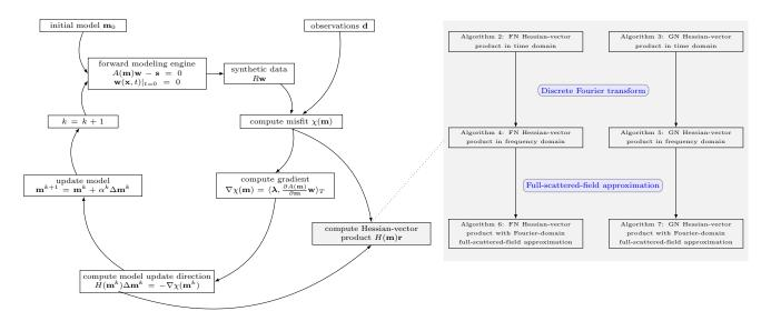
Figure 1: A brief workflow of the truncated Newton method. Note that the vector  $\mathbf{r}$  used in Hessian-vector product construction is given by the CG algorithm during solving the Newton equation.
