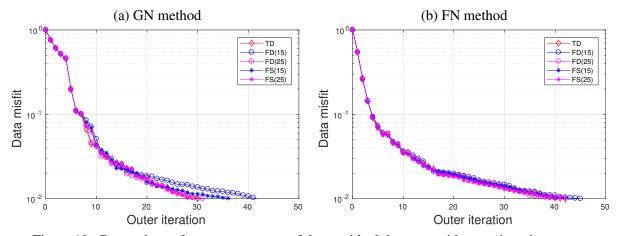
Figure 10: Comparison of convergence rate of data residual decrease with outer iteration.
