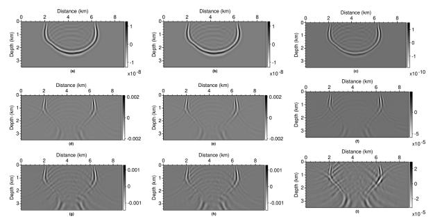
Figure 6: Comparison of the wavefields between first-order Born modeling (left column) and full-scattered-field approximation (middle column) using snapshots at t=1.5s, and the corresponding differences are presented in the right column: second-order incident wavefields  ${\bf u}$  (first row), second-order adjoint wavefields in GN method  ${\boldsymbol \mu}_1$ , and second-order adjoint wavefields in FN method  ${\boldsymbol \mu}_L$ .
