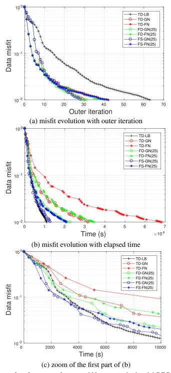
Figure 12: Comparison of performance of truncated Newton method and  $\ell$ -BFGS method. Truncated Newton methods have a faster iterative convergence rate over  $\ell$ -BFGS method. With two approximations, the proposed truncated Newton methods can provide a competitive elapsed-time convergence rate with  $\ell$ -BFGS method.
