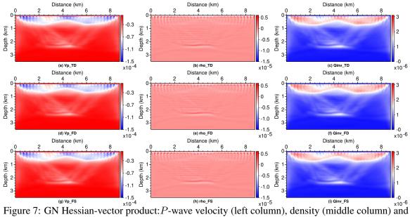
Figure 7: GN Hessian-vector product: P-wave velocity (left column), density (middle column) and  $Q^{-1}$  (right column). Time-domain implementation (first row), frequency-domain approximation (second row) and full-scattered-field approach in frequency domain (third row). 25 frequencies are used in two approximate methods.
