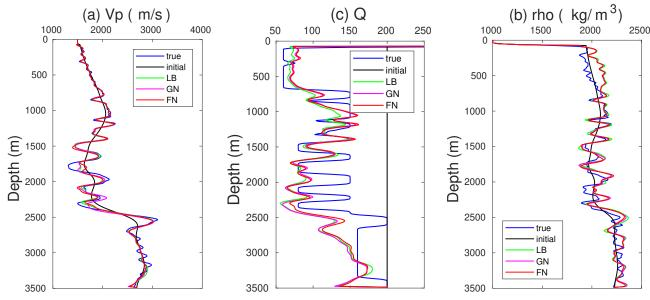
Figure 16: The extracted vertical profiles from final inverted velocity, density, and Q at the distance x=4 km. The results of truncated Newton method are obtained with Fourier-domain full-scattered-field approximation.
