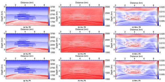
Figure 13: Final inversion results with truncated GN method: P-wave velocity (left column), density (middle column) and  $Q^{-1}$  (right column). Time-domain implementation (first row), frequency-domain approximation (second row) and full-scattered-field approach in frequency domain (third row). 25 frequencies are used in two approximate methods.
