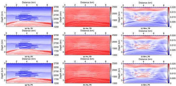
Figure 14: Final inversion results with truncated FN method: P-wave velocity (left column), density (middle column) and  $Q^{-1}$  (right column). Time-domain implementation (first row), frequency-domain approximation (second row) and full-scattered-field approach in frequency domain (third row). 25 frequencies are used in two approximate methods.
