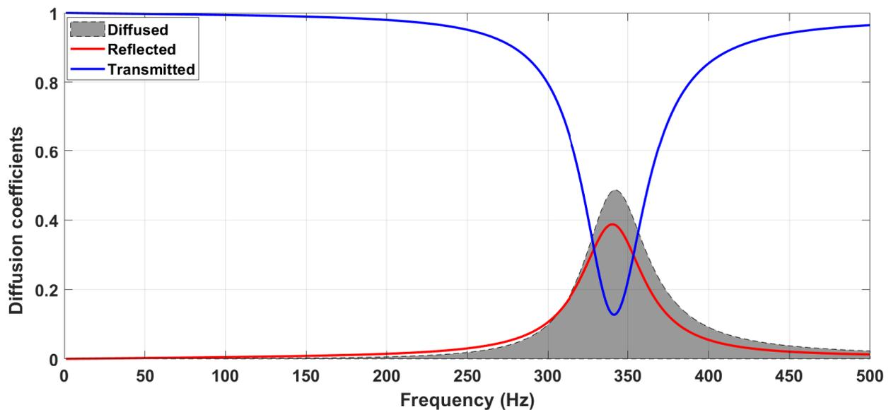
Figure 7: Diffused, reflected and transmitted waves through the resonator's coupling element.
