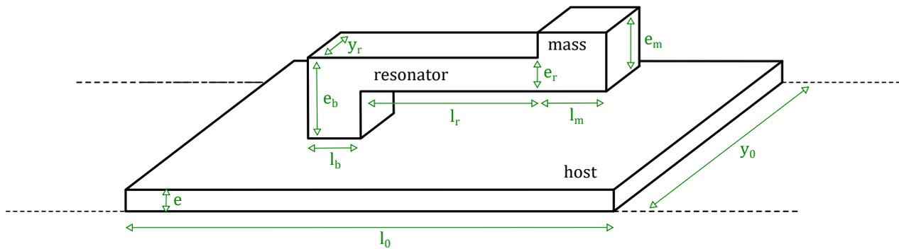
Figure 1: Description of the periodic unit-cell use for Bloch analyses.
