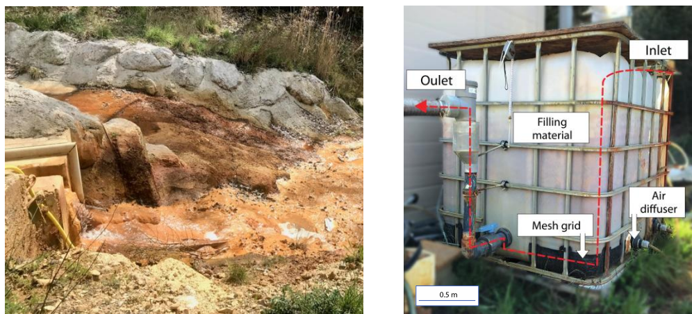
Figure 1. AMD stream and treatment device in-situ (polyethylene container).
