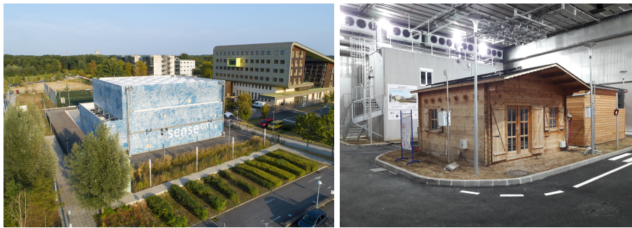
Figure 1: View of the climatic chamber (left) and the mini-city 1 covered by the climatic chamber (right)
