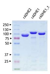
**Fig. 3**. SDS-PAGE analysis of recombinant *Polytomella* ADHEs. Proteins purified by affinity chromatography ( $10 \mu G$ ) were separated on a 10% acrylamide gel and stained with Coomassie Brilliant Blue R. rADHE2, recombinant ADHE1; rADHE1\_t, recombinant ADHE1 lacking its 41 carboxy-terminal residues. The gel is representative of three independent protein purifications.
