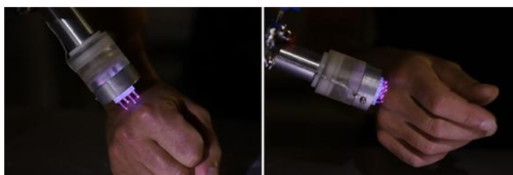
Figure 2 Top: schematic of the low voltage multi-jet applicator (option 3). Bottom: 4 and 9 low voltage multi-jets delivered on the author's hand. Parameters: voltage 2.5 kV, repetition rate 20 kHz, gas flow 2 L/min.
