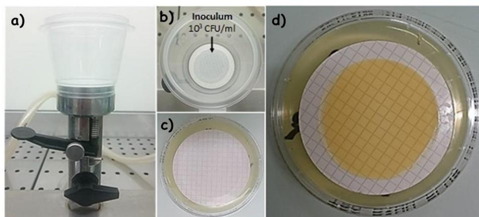
**Figure 3** a) Funnel and valve connected to a vacuum pump (not shown) used to initiate the bacteria inoculum preparation, b) Top view of funnel, whose base is covered with a membrane used to filter the bacterial inoculum, c) zoom on the membrane set on agar prepared in a petri dish right at the end of the filtering process, d) view of the grown bacterial lawn following a 24-hour incubation at  $37^\circ\text{C}$ .
