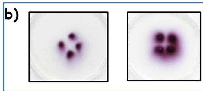
**Figure 6** a) Current delivered on a metallic target with 4 jets: bold black trace, 3 jets thin grey trace, 2 jets: bold grey trace and 1 jet: thin black trace, b) image of KI-enriched agar samples exposed to four multi-jets generated with the low voltage applicator during left: 60 s and right: 240 s.
