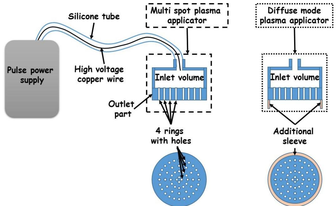
**Figure 1** Schematic of the multi-jets devices (option 2) with pulse power supply, high voltage wire inside the silicone and center: multi-spot, and right: diffuse mode applicators. On bottom end on view of the applicators. When operated, the silicone tube connection for the diffuse mode applicator is the same as for the multi-spot applicator.
