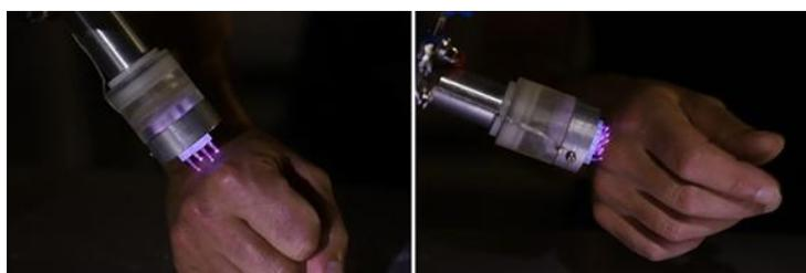
**Figure 2** Top: schematic of the low voltage multi-jet applicator (option 3). Bottom: 4 and 9 low voltage multi-jets delivered on the author's hand. Parameters: voltage 2.5 kV, repetition rate 20 kHz, gas flow 2 L/min.
