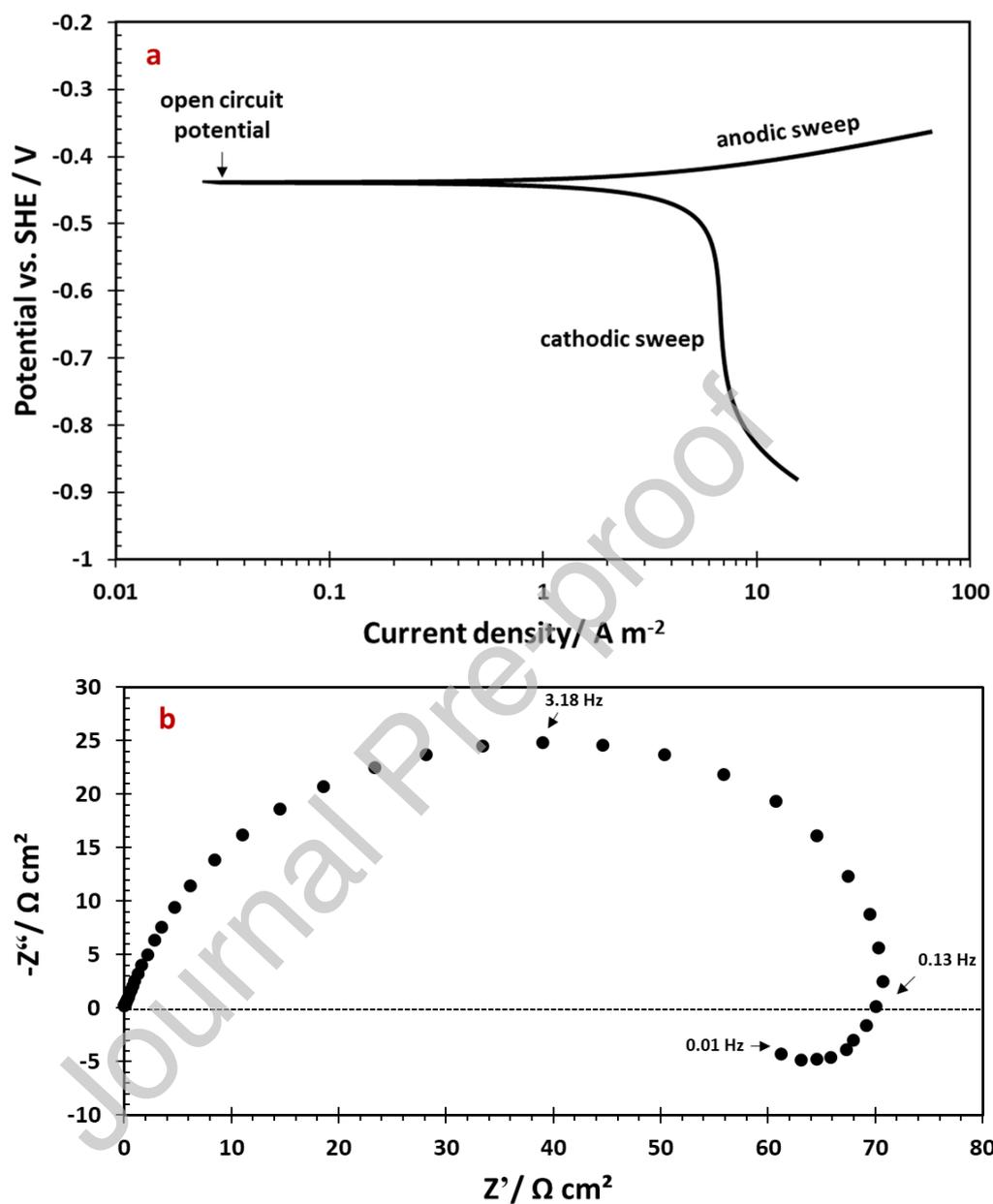
Figure 1. Corrosion of X65 mild steel RDE @ 2000 rpm, 0.1 M NaCl aqueous solution sparged with 1 bar CO<sub>2</sub>, pH 4.0, 30 °C; a) steady state potentiodynamic polarization sweeps; b) electrochemical impedance spectrum conducted at the open circuit potential (OCP) shown as a Nyquist plot.
