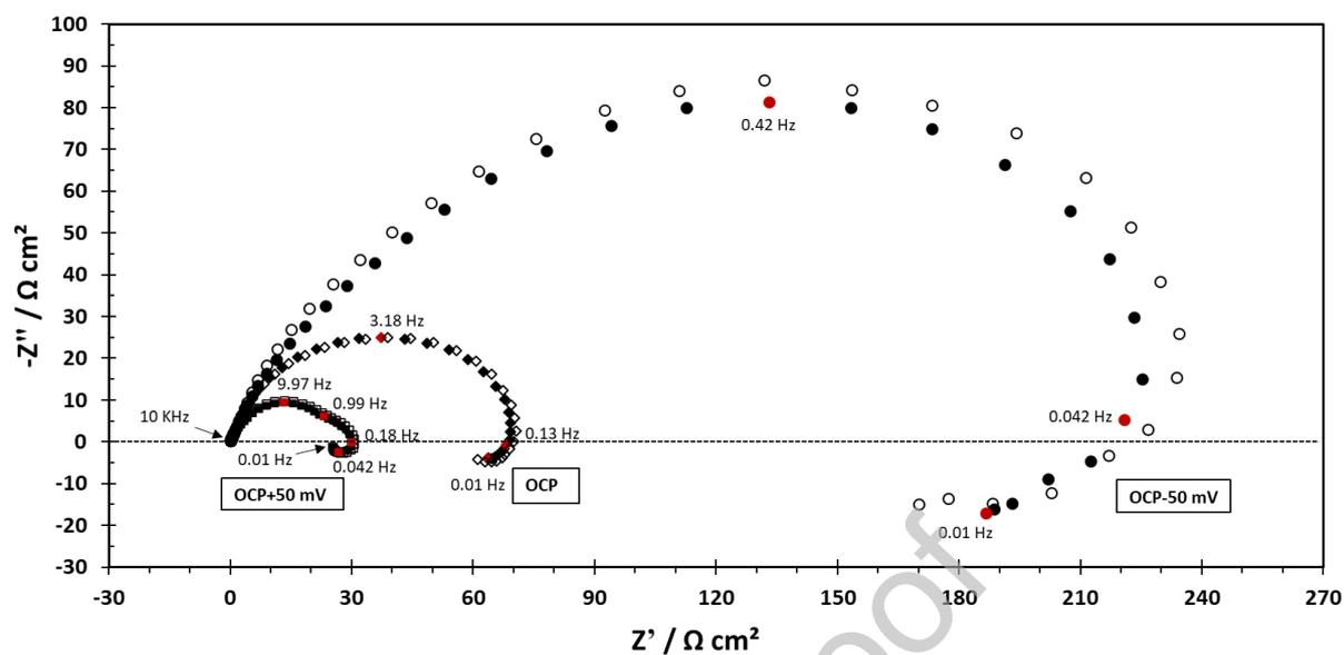
Figure 8. Nyquist plot at OCP + 50 mV, OCP, and OCP – 50 mV. Experimental parameters: X65 mild steel RDE, 2000 rpm, pH 4.0, 30 °C, aqueous solution saturated at 1 bar CO<sub>2</sub>, 0.1 M NaCl supporting electrolyte and frequency range from 10,000 - 0.01 Hz. Nyquist plots having the same shaped markers represents duplicated experiments.
