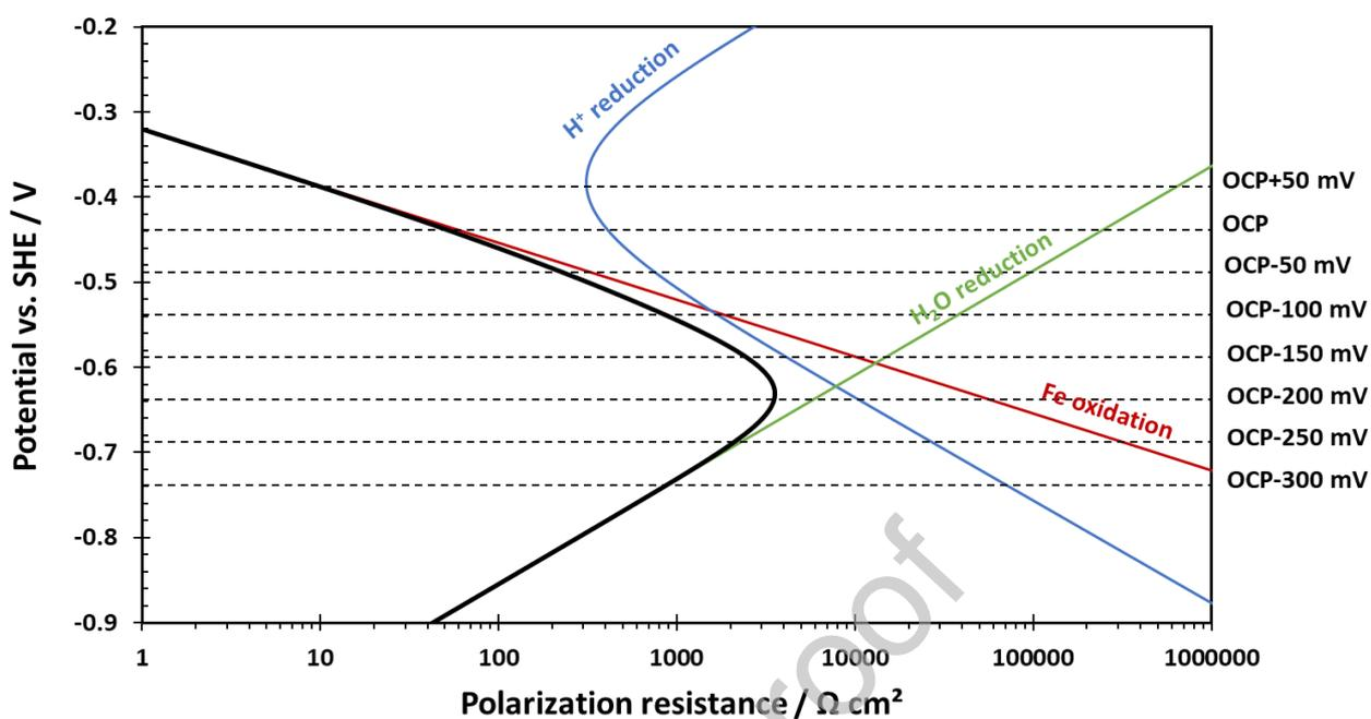
Figure 6. Modeled polarization resistance of  $\text{H}^+$  reduction, Fe oxidation,  $\text{H}_2\text{O}$  reduction and overall polarization resistance, derived from the modeled potentiodynamic sweeps shown in Figure 4. Modeling parameters: X65 mild steel RDE, 2000 rpm, pH 4.0, 30 °C, aqueous solution saturated at 1 bar  $\text{CO}_2$ , and with 0.1 M NaCl supporting electrolyte.
