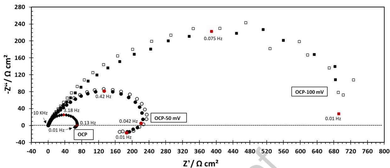
Figure 9. Nyquist plot at different OCP, OCP – 50 mV and OCP – 100 mV. Experimental parameters: X65 mild steel RDE, 2000 rpm, pH 4.0, 30 °C, aqueous solution saturated at 1 bar CO<sub>2</sub>, 0.1 M NaCl supporting electrolyte and frequency range from 10,000 - 0.01 Hz. Nyquist plots having the same shaped markers represents duplicated experiments.
