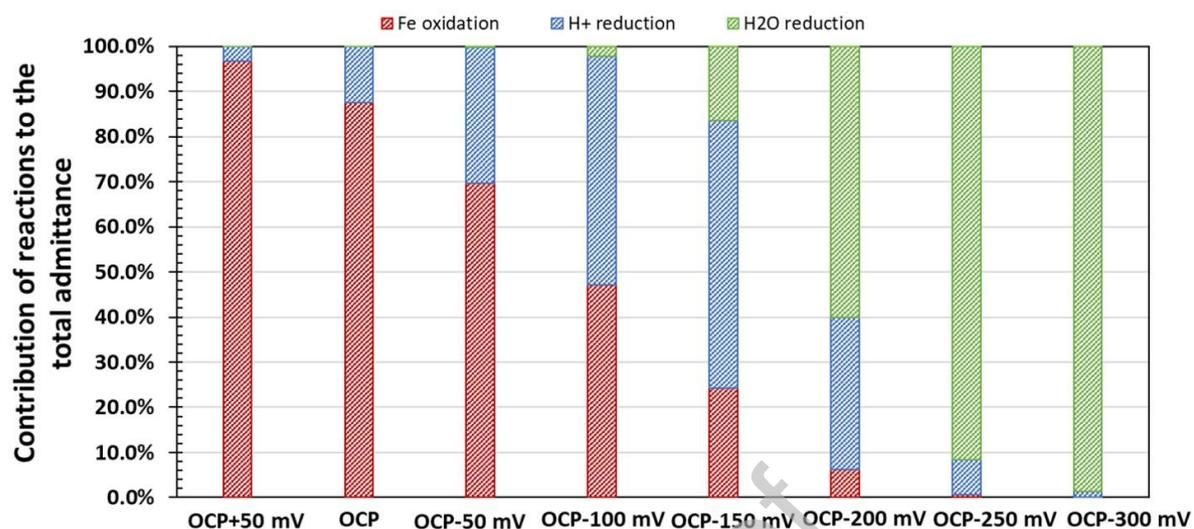
Figure 7. Contribution of individual reaction ( $\text{H}^+$  reduction, Fe oxidation and  $\text{H}_2\text{O}$  reduction) to the total admittance, based on Figure 6. Modeling parameters: X65 mild steel RDE, 2000 rpm, pH 4.0, 30 °C, aqueous solution saturated at 1 bar  $\text{CO}_2$ , and with 0.1 M NaCl supporting electrolyte.
