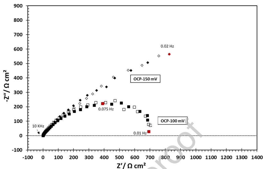
Figure 10. Nyquist plot at different OCP – 100 mV and OCP – 150 mV. Experimental parameters: X65 mild steel RDE, 2000 rpm, pH 4.0, 30 °C, aqueous solution saturated at 1 bar CO<sub>2</sub>, 0.1 M NaCl supporting electrolyte and frequency range from 10,000 - 0.01 Hz. Nyquist plots having the same shaped markers represents duplicated experiments.
