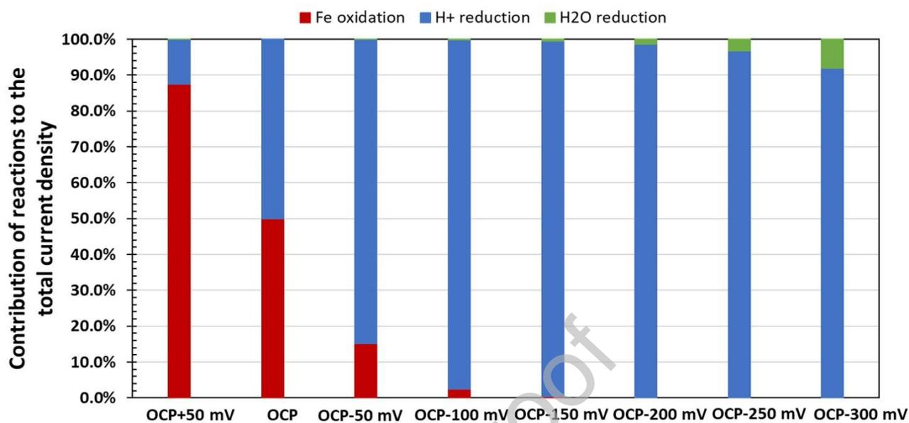
Figure 5. Contribution of each reaction ( $\text{H}^+$  reduction, Fe oxidation and  $\text{H}_2\text{O}$  reduction) to the total current density, based on Figure 4. Modeling parameters: X65 mild steel RDE, 2000 rpm, pH 4.0, 30 °C, aqueous solution saturated at 1 bar  $\text{CO}_2$ , and with 0.1 M NaCl supporting electrolyte.
