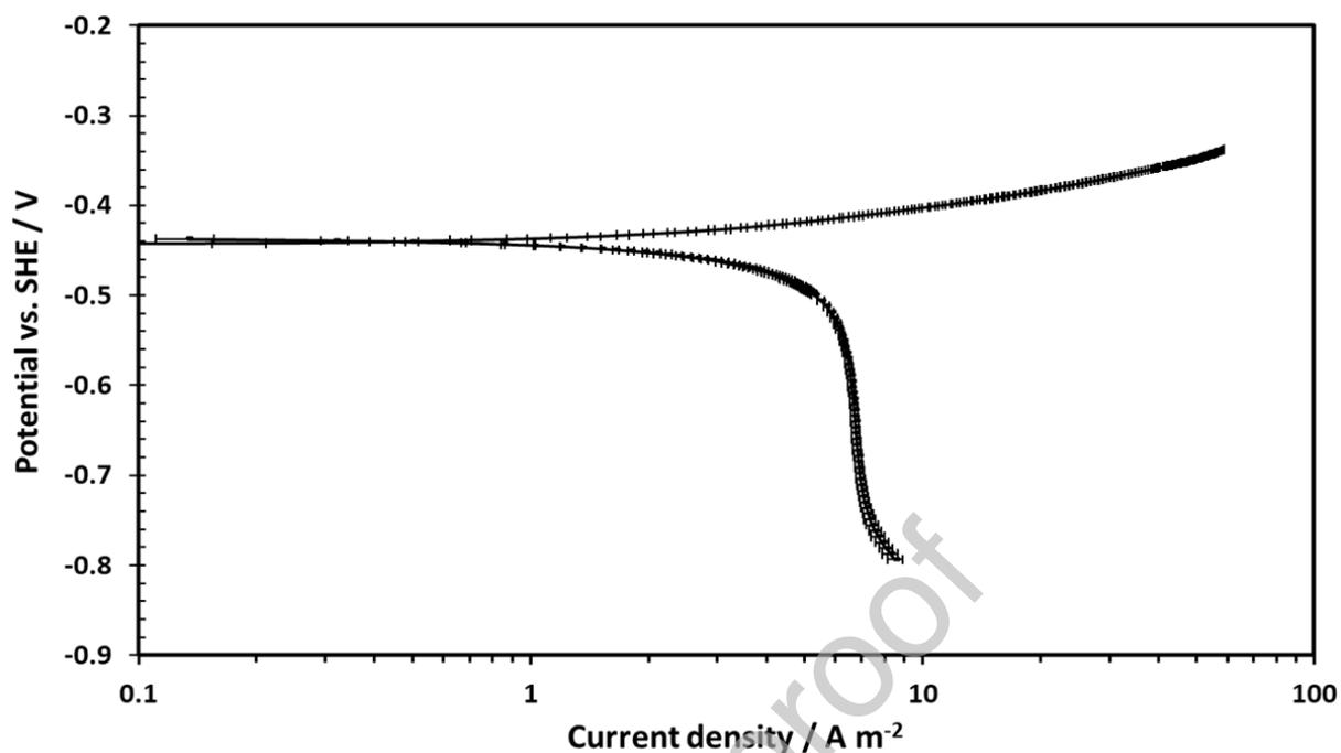
Figure 3. Steady state polarization sweep curve, measured using a sweep rate of  $0.125 \text{ mV s}^{-1}$ , on X65 mild steel RDE at 2000 rpm, corroding in an aqueous solution at pH 4.0,  $30 \text{ }^\circ\text{C}$ , saturated at 1 bar  $\text{CO}_2$ , with 0.1 M NaCl supporting electrolyte. Error bars represent minimum and maximum current densities calculated in duplicated experiments.
