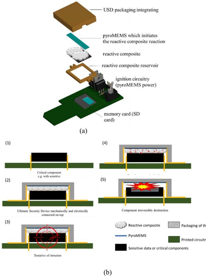
**Figure 1.** Conceptual illustration of the USD operation principle. (a) Exploded view of the device, composed of a 2 stacked parts (a pyroMEMS and reactive composite printed in a reservoir). (b) Operating mechanism for utilizing the USD as a protecting device against the intrusion of data contained in a memory.
