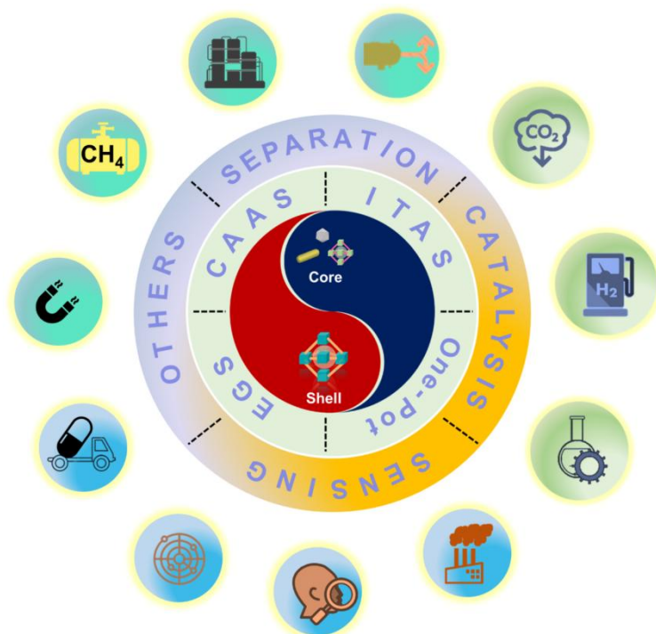
Scheme 1. Illustration of the synthetic methods (CAAS = Capping agent-assisted synthesis; ITAS = Inorganic template-assisted synthesis; EGS = Epitaxial growth synthesis) and the main applications of core-shell MOFs based composites.
