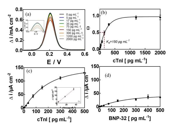
**Figure 3.** (A) Differential pulse voltammograms for different cTnI concentrations (0, 5, 17, 35, 75, 150, 300, 1200 and 2000 pg mL<sup>-1</sup>) in 1 × PBS (pH 7.4) without washing steps. (b) Langmuir model of cTnI binding extracted form Figure 3a as a function of the analyte concentration of the solution running through the flow cell. (c) Calibration curve of CTnI in 1x PBS (pH 7.4). (d) Calibration curve of BNP-32 1 × PBS (pH 7.4) on CTnI apatamer modified electrode.
