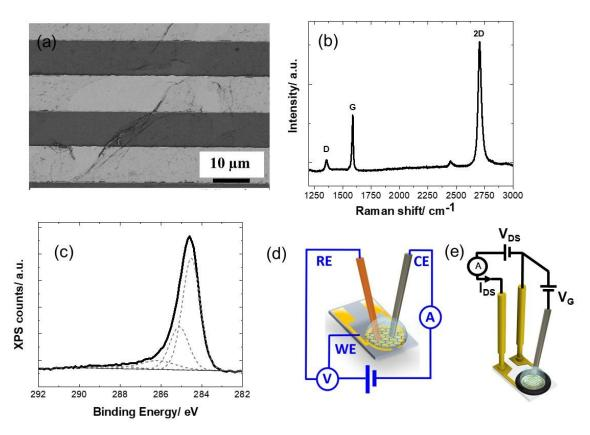
**Figure 1. Characterization of graphene-based electrodes for electrochemical surface modification and sensing**: (a) SEM image of the IDE chip after coating with CVD graphene showing full coverage over the gold lines as well as the space between IDE. (b) Raman spectrum of the graphene channel. (e) C1s core level spectrum of the electrode. (d) Scheme of
