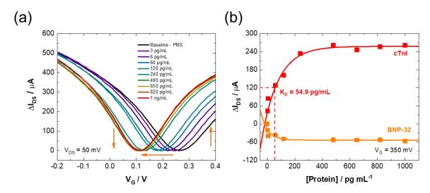
**Figure 4:** (a) Graphene transfer characteristics in  $0.01 \times$  PBS (pH 7.4) without washing steps for different cTnI concentrations. Applied  $V_{DS} = 50$  mV. (b)  $\Delta I_{DS}$  for each cTnI concentration (red curve) and BNP-32 concentration (orange curve) at a fixed gate voltage  $V_G = 350$  mV with respective Langmuir binding isotherm and estimated  $K_D$ .
