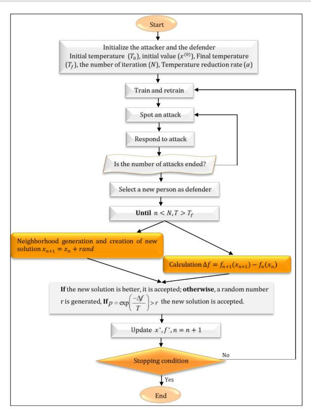
Figure 8: The flowchart of HSEOSA.
