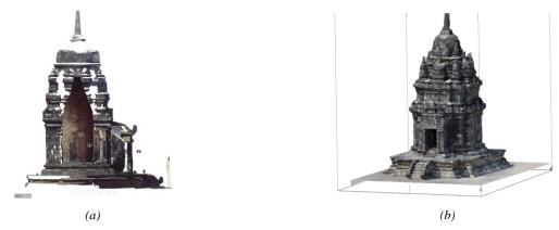
**Figure 3.** A sample of results from the tropical school as created by the participants: (a) laser scan of a shrine interior and (b) photogrammetic point cloud of the same shrine's exterior. Note that to each group one shrine was attributed.
