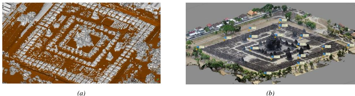
**Figure 4.** Some results of the documentation project and technical demonstrations: (a) lidar point cloud classified into ground and non-ground classes, (b) georeferenced drone photogrammetric point cloud.
