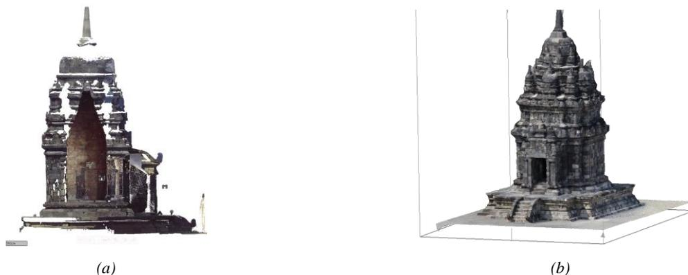
**Figure 3.** A sample of results from the tropical school as created by the participants: (a) laser scan of a shrine interior and (b) photogrammetric point cloud of the same shrine's exterior. Note that to each group one shrine was attributed.
