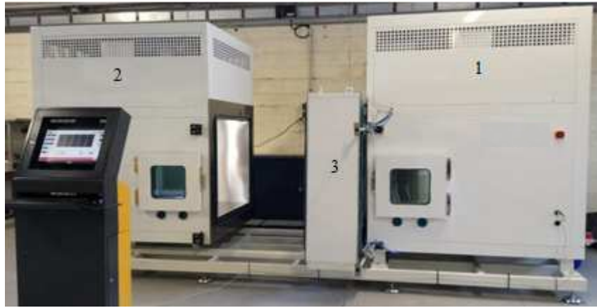
Figure 3: Test bench (1: indoor climatic room, 2: outdoor climatic room, 3: wall sample holder).
