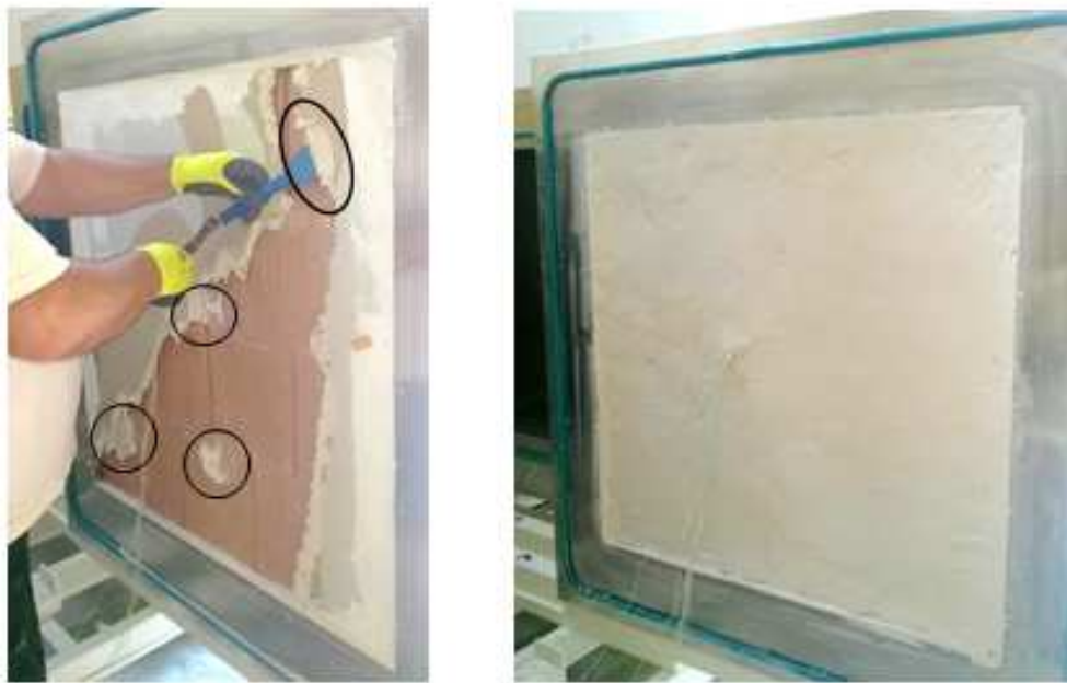
Figure 19: Plasterboard wall sample with glue points highlight (left) and plaster coating wall sample (right).
