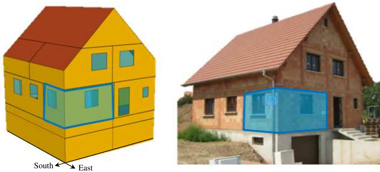
Figure 10: Studied residential building perspective (TRNSYS 3D on left with instrumented room in blue).
