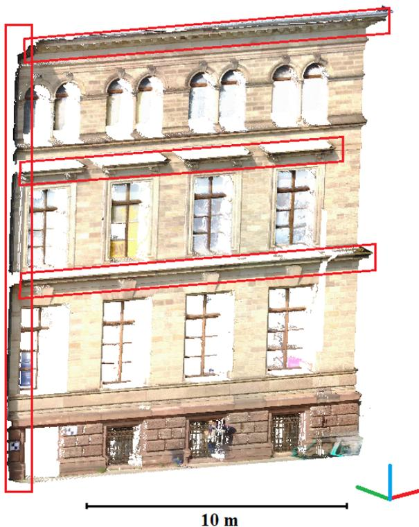
(a) Point cloud of a part of the façade acquired from one scan station (colorized with RGB values)
