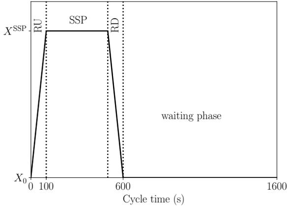
Figure 2: Evolution of the quantity  $X$  ( $\phi_{\text{ion}}$ ,  $E_{\text{ion}}$ ,  $T_{\text{surf}}$ ) during a 1600-seconds cycle, from its lowest value  $X_0$  during the waiting phase to its highest value during the steady-state plasma (SSP). RU = Ramp-up, RD = Ramp-down.
