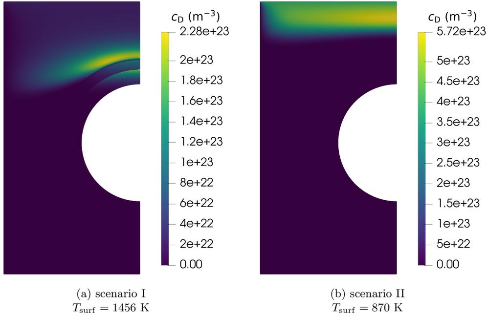
Figure 7: Results of the FESTIM simulations for scenario I (a) and II (b): deuterium retention field  $c_D$  ( $\text{m}^{-3}$ ), in the semi-monoblock after 10,000 seconds of continuous. The colour bar have different scales .
