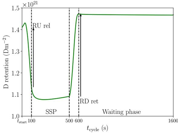
Figure 5: Evolution of the D retention with time during the 10<sup>th</sup> cycle of scenario II ( $T_{\text{surf}}^{\text{SSP}} = 870$  K). The beginning/end of the plasma ramp-up/down are marked with vertical dashed line and the retention released during the ramp-up (RU rel) and retained during the ramp down (RD ret) are marked with arrow.
