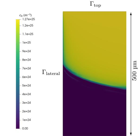
Figure 8: Results of the FESTIM simulation for the scenario III: deuterium retention field  $c_D$  ( $\text{m}^{-3}$ ) after 10,000 second of continuous plasma exposure (on  $\Gamma_{\text{top}}$ ). The thickness of the simulated material is 500  $\mu\text{m}$ . The width is the same as for the other scenarios (14 mm) but for sake of clarity, the figure is zoomed in the corner from which the D is allow to desorb ( $\Gamma_{\text{lateral}}$ ). The temperature is 435 K.
