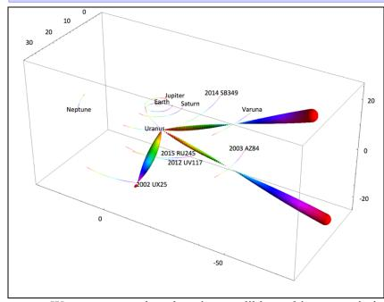
Figure 2: Three possible TNO flyby trajectories after a Uranus flyby, illustrating the wealth of options for TNO exploration from one pre-Uranus mission architecture. Search volumes appear as colored spheres, distributed spacecraft along the trajectories after Uranus encounter, with the color scale resetting at that point and running for 20 years. The narrowing of the search volumes to zero radius indicate locations of primary TNO target encounters. [72]
