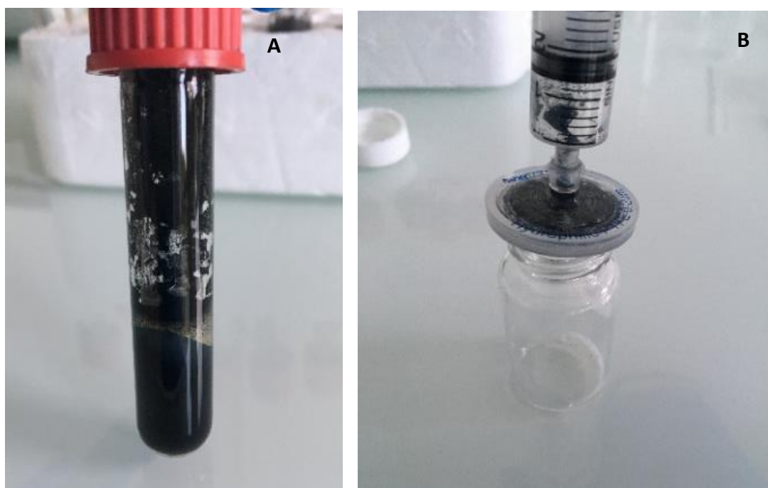
Low density GBMs in HBS after centrifugation, 10 g/L concentration (A) and filtration (B). Please note that the filtrate should be clear.
