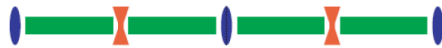
FIG. 15. FODO sketch: Focusing and defocusing quadrupoles placed in between the undulator segments.
