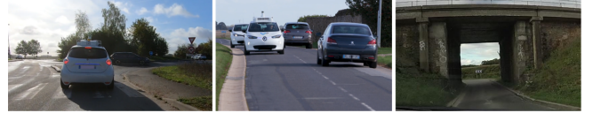
Fig. 1. Tornado project key scenarios demonstration. Left graphic corresponds to a roundabout entrance. Centre graphic depicts a narrow two-way road with a gutter. Right graphic plots a non-visibility tunnel crossing with a reduction from two-way to a single lane.
