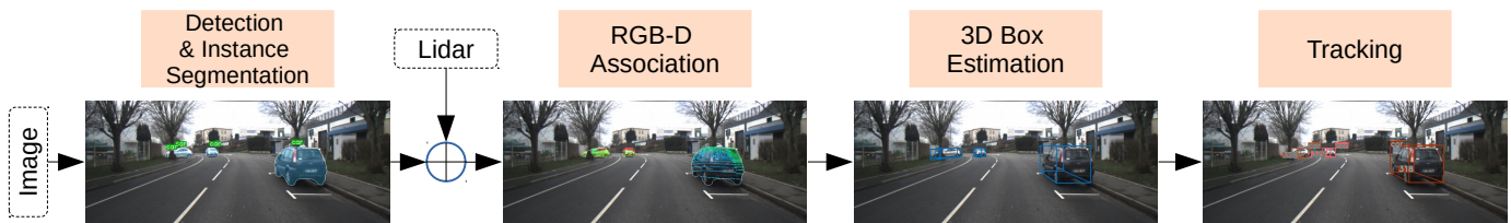
Fig. 4. Pipeline for 3D object detection. Objects are detected in the images from the cameras. Later, LiDAR data is included to infer the geometrical properties of the objects. Finally, all the detections are merged, and a tracking stage adds temporal consistency across consecutive frames.
