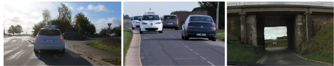
Fig. 1. Tornado project key scenarios demonstration. Left graphic corresponds to a roundabout entrance. Centre graphic depicts a narrow two-way road with a gutter. Right graphic plots a non-visibility tunnel crossing with a reduction from two-way to a single lane.
