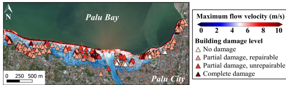
Figure C3. Sulawesi–Palu final tsunami inundation model with the maximum simulated flow velocity overlaid on the damaged building data (background ESRI).
