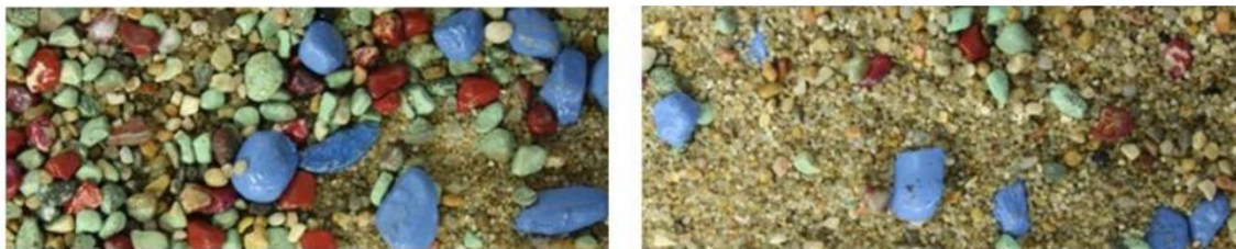
Figure 2 : a) Congested (armor) and b) smooth bed (no armor)
