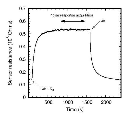
Fig. 3. Example of a response of studied WO<sub>3</sub> gas sensor under 80ppb ozone (O<sub>3</sub>) concentration.
