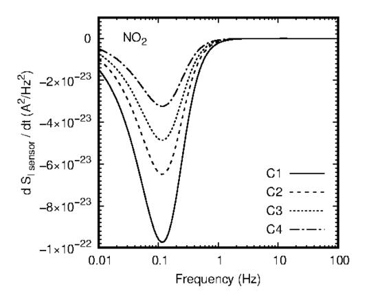
Fig. 5. Plots of the first derivtive of noise current spectral density for the four concentrations of nitrogen dioxide.
