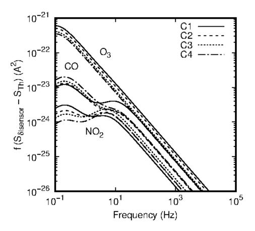
Fig. 6. Plots of the quantity  $f \cdot (S_{\mathcal{A}_{sensor}}(f) - S_{Th}(f))$  for four concentrations of ozone (O<sub>3</sub>), nitrogen dioxide (NO<sub>2</sub>) and carbon monoxide (CO) detected by metal-oxide gas microsensor with tungsten trioxide (WO<sub>3</sub>) sensing layer.
