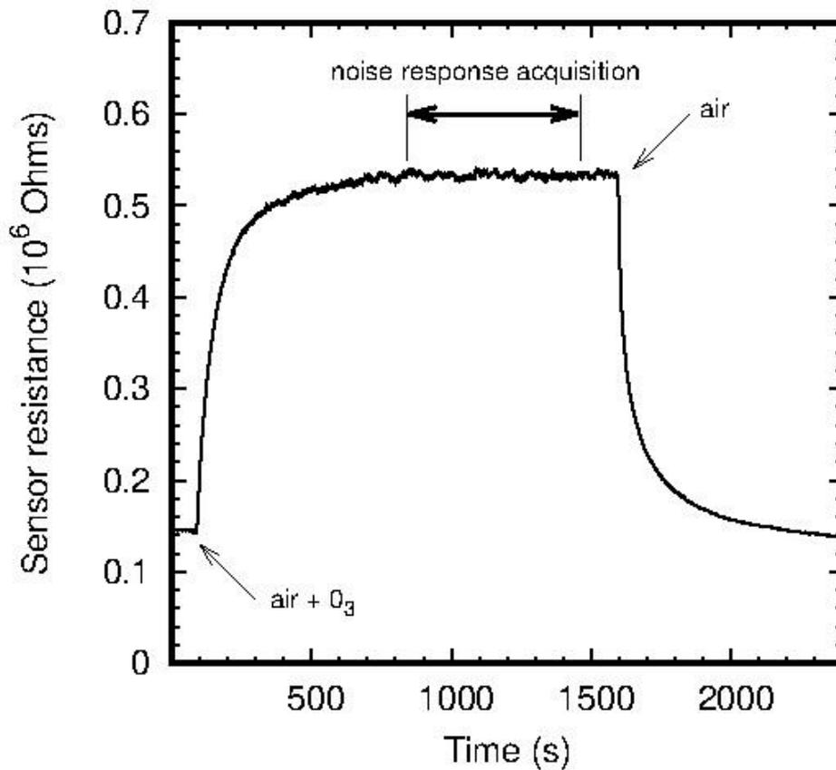
Fig. 3. Example of a response of studied  $\text{WO}_3$  gas sensor under 80ppb ozone ( $\text{O}_3$ ) concentration.
