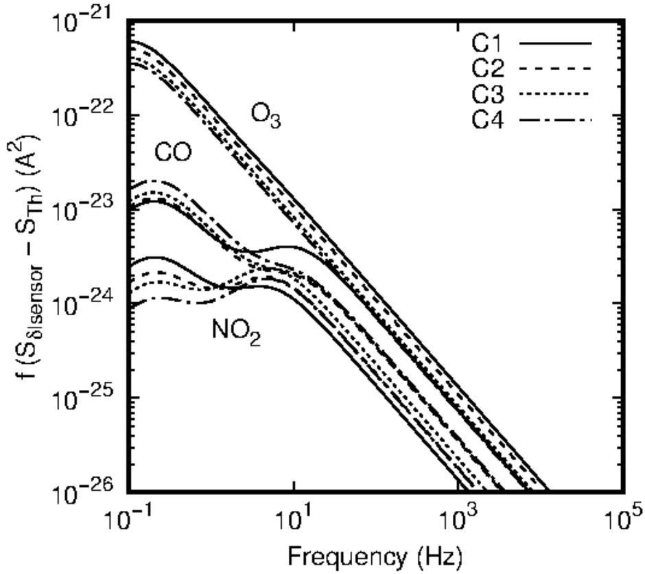
Fig. 6. Plots of the quantity  $f \cdot (S_{\delta_{\text{sensor}}}(f) - S_{Th}(f))$  for four concentrations of ozone ( $O_3$ ), nitrogen dioxide ( $NO_2$ ) and carbon monoxide (CO) detected by metal-oxide gas microsensor with tungsten trioxide ( $WO_3$ ) sensing layer.
