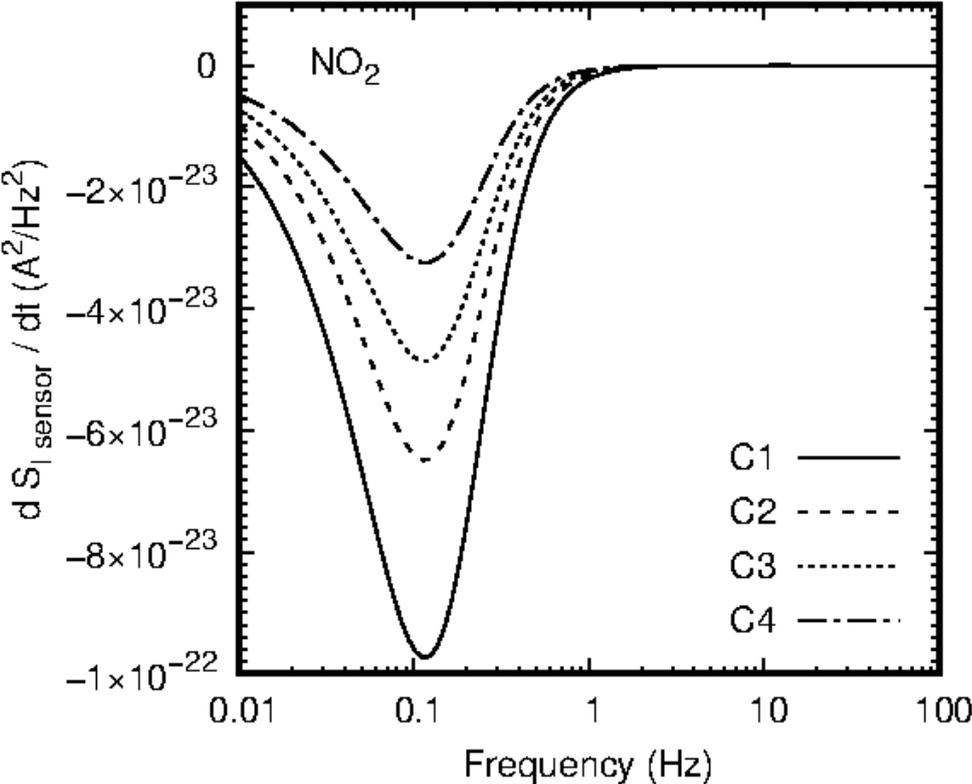
Fig. 5. Plots of the first derivative of noise current spectral density for the four concentrations of nitrogen dioxide.
