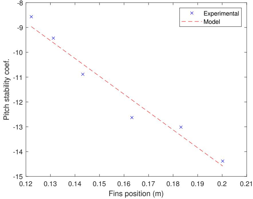
**Fig. 4**  $Cm_\alpha$  metamodel fit on identification data
