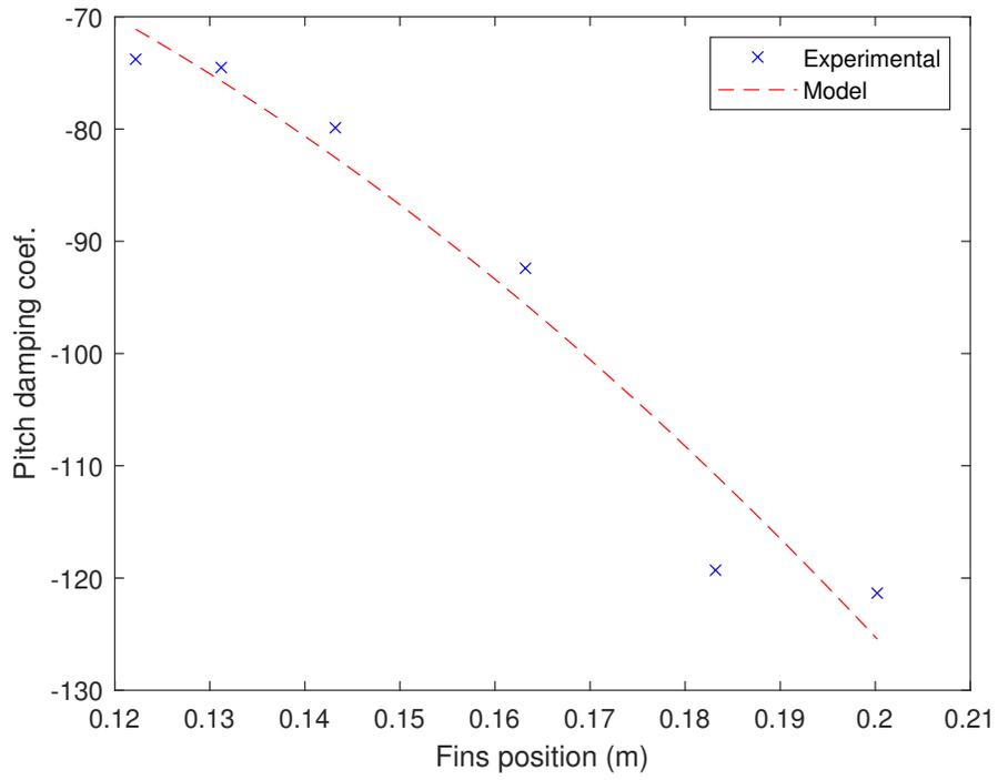
**Fig. 5**  $Cm_q$  metamodel fit on identification data
