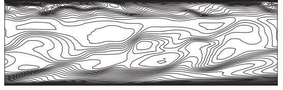
Figure 2: Contours of the instantaneous passive scalar in the (x_1, x_3) mid-plane illustrating the unsteady character of the scalar field. P_r = 1 .
