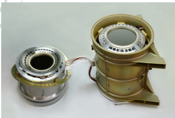
1967 1968 1969 1970 1971 1972 1973 1974 1975 1976 1977 1978 1979 Fig. 41 Copper sulfide blackened energy analyzer (left) and entrance section (right)
