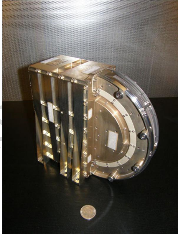
Fig. 73 ENA flight model. The sensor is wrapped by MLI, when ENA is installed in the spacecraft
