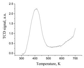
Fig. 3 CO<sub>2</sub>-TPD profile of the prepared carbon nitride (C<sub>3</sub>N<sub>4</sub>-bulk).
