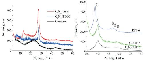
Fig. 1 X-ray diffraction patterns of the prepared supports: left: carbon nitride and microporous carbon; right: initial silica MMS KIT-6, C<sub>x</sub>N<sub>y</sub>-KIT-6 and C-KIT-6.
