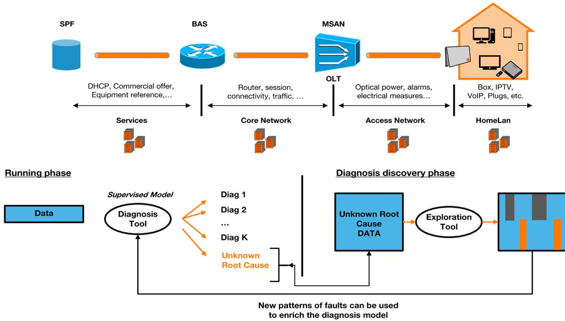
**FIGURE 1.** Illustration of the diagnosis process and its application to FTTH network services. Where, SPF: Service Platform; DHCP: Dynamic Host Control Protocol; BAS: Broadband Access Server; MSAN: Multi-Service Access Node; OLT: Optical Line Termination; Home LAN: Home Local Area Network; VoIP: Voice over IP.
