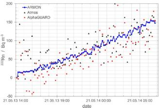
**Figure 7.** A preliminary low-level comparison between ARMON (in blue) and two commercial monitors (ATMOS and AlphaGUARD) (in black and red) carried out within the INTE-UPC radon chamber during an activity concentration build-up phase. INTE-UPC operates a radon chamber, categorized as a STAR according to [55].
