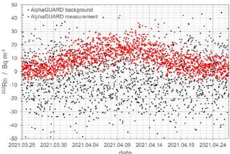
**Figure 3.** A low-level calibration situation in a non-constant atmosphere: One AlphaGuard in red from figure 2 in a build-up and decay situation in a closed large volume climate chamber at PTB. The activity concentration outside the climate chamber is given by a second AlphaGuard in black.
