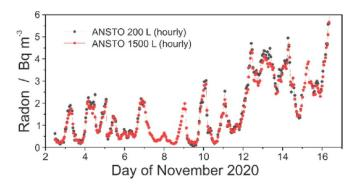
**Figure 6.** Two-week comparison of hourly atmospheric radon activity concentration observations between a 200 l and 1500 l ANSTO radon detector from 3 m above ground level at a site near Sydney, Australia, 15 km from the coast.
