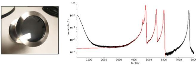
**Figure 1.** The integrated source-detection system: on the left, an ion-implanted silicon semiconductor detector, coated in a defined manner with  $^{226}\text{RaCl}_2$  by means of thermal vapor deposition; on the right, the resulting  $\alpha$ -spectrum. The respective peaks are well resolved. For the tailing contributions a model with mixtures of exponentially modified Gaussians is used. © Physikalisch-Technische Bundesanstalt.
