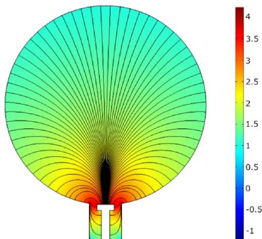
**Figure 8.** Upper part: simulation of the electric field ( $\text{kV m}^{-1}$ ) generated within the detection volume of the ARMON v2; Bottom part: user Interface of the ARMON v2.
