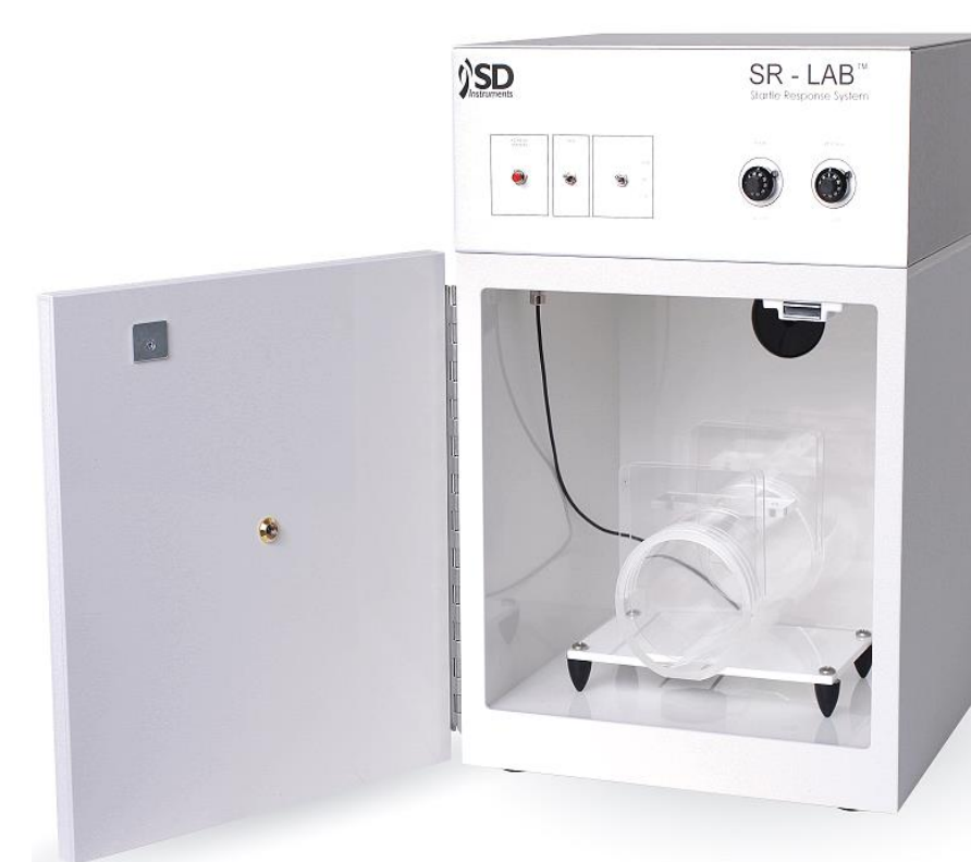
Figure 4. Apparatus for measurement of the ASR in mice. Animals were presented with pulses of white sound of 20 ms duration and varying intensity: +6, +12 +18 and +24 dB over the 66dB bckgd level.
