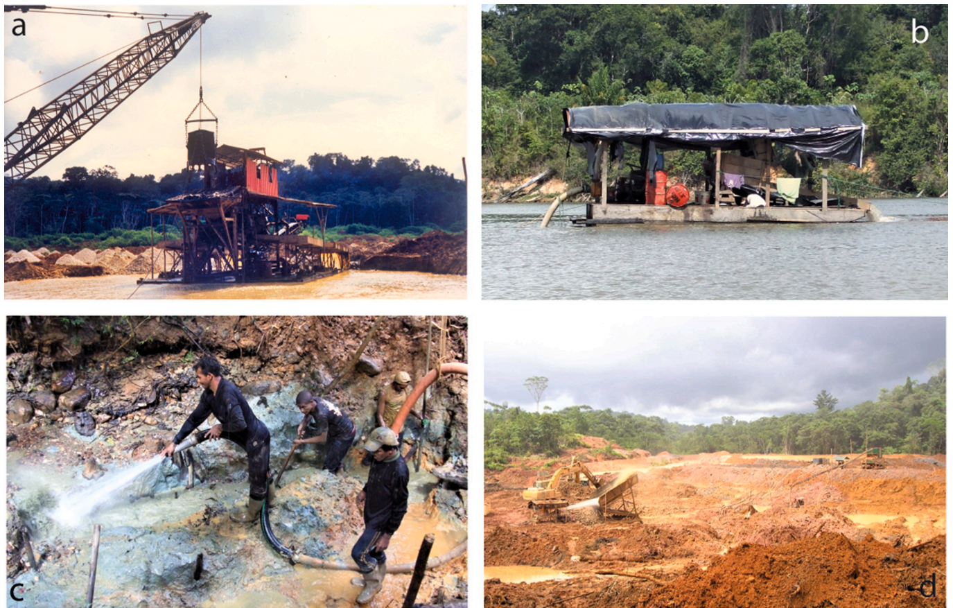
Fig. 6. Gold mining techniques used in French Guiana after WWII. a) Bodinson floating plant and American dragline, Crique Roche, Paul Isnard (Compagnie Minière de Paul Isnard; P. Rostan Collection); b) Suction dredge on the Awa River. This procedure, banned in French Guiana since 1996, is still used in Suriname (2008, Benzdorp; photograph P. Rostan); c) Illegal Brazilian miners monitoring a gravel pump (2008, Crique Roche, Saül, photograph P. Rostan); d) Modern alluvial exploitation showing an excavator, gravel pump, screen with bars (“grizzly”) and gold mat (2007, Boulanger Creek; photograph P. Rostan).
