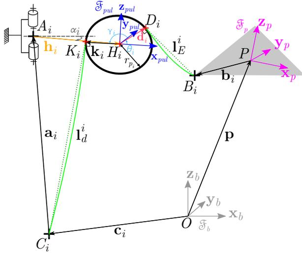
Figure 1:  $CDPR_{SR}$  parametrization with single revolute joint pulleys
