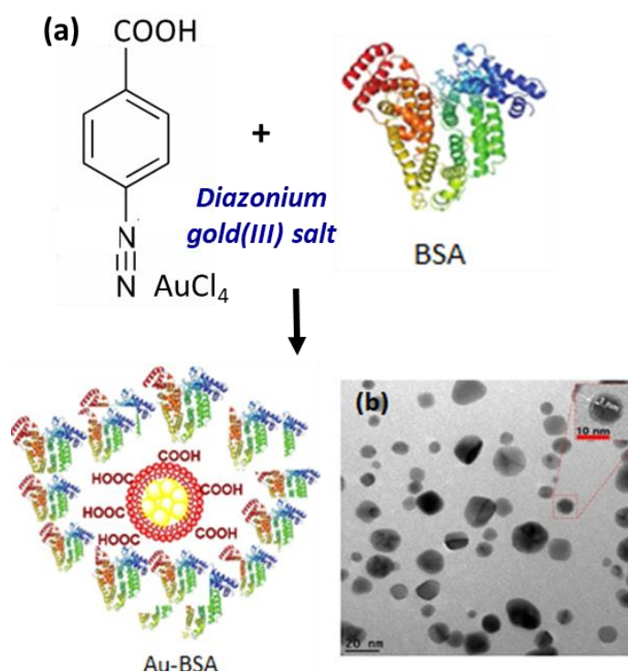
Figure 4. (a) Synthesis of Au NPs directly capped with aryl groups derived from diazonium salts and coated with BSA. (b) TEM image of Au NPs-BSA bioconjugates. The inset evidences the presence of the BSA layer. Reproduced with permission from ref. 78. Copyright, 2018 Elsevier.
