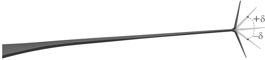
Figure 2: Active winglet principle with variable cant angle.
