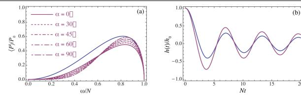
FIG. 2 – For a circular cylinder (——) and a sphere (——), (a) power output of forced oscillations, normalized by  $P_0 = \rho_0 N^3 a^2 A^2$  for the cylinder and  $\rho_0 N^3 a^3 A^2$  for the sphere, and (b) free buoyant oscillations.
