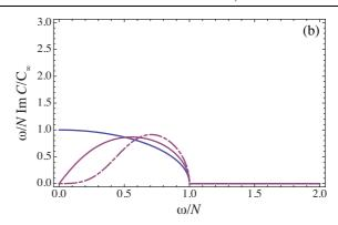
FIG. 1 – Coefficients of (a) added mass and (b) damping for a circular cylinder (——) and a sphere oscillating either vertically (——) or horizontally (———).
