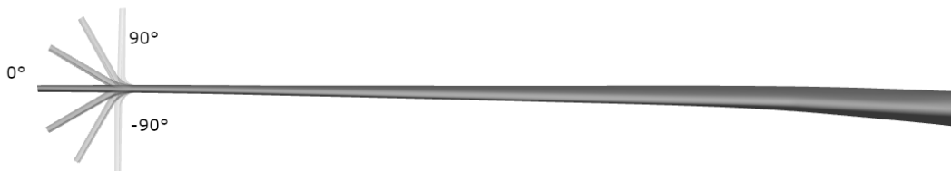
Fig. 2 XRF1 high AR wing with various cant angle deflections of the wing-tip
