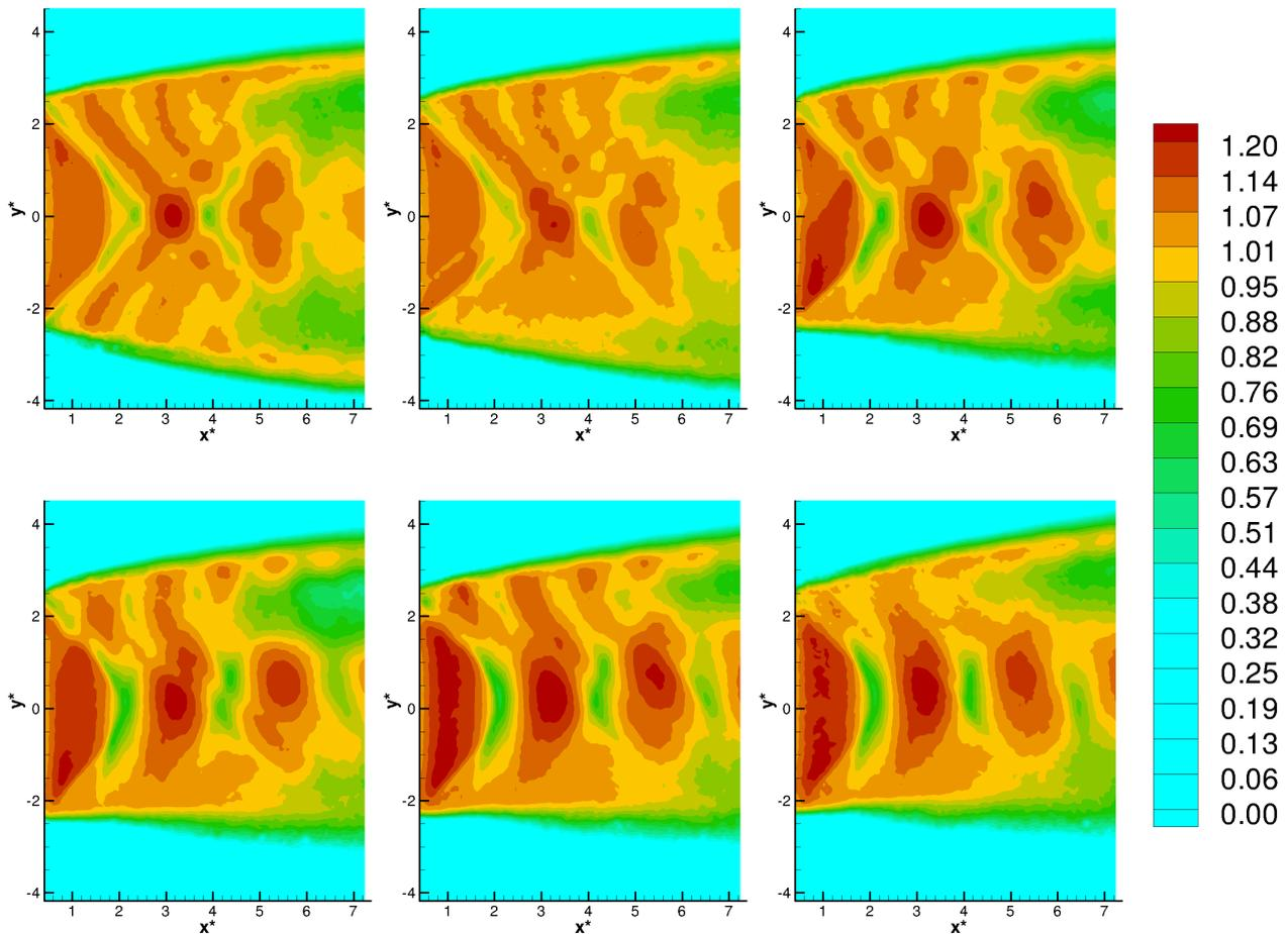
Figure 7: Iso-contours of of mean axial velocity  $U^*$  downstream of the nozzle, from left to right and top to bottom :  $\Delta Q = 0\%$ ,  $\Delta Q = 0.31\%$ ,  $\Delta Q = 0.63\%$ ,  $\Delta Q = 1.0\%$ ,  $\Delta Q = 1.3\%$ ,  $\Delta Q = 1.62\%$
