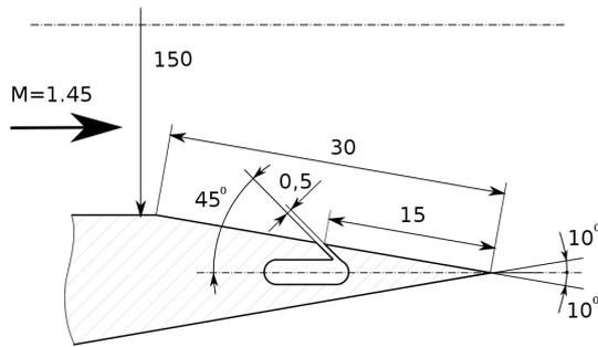
Figure 1: Divergent and actuator
