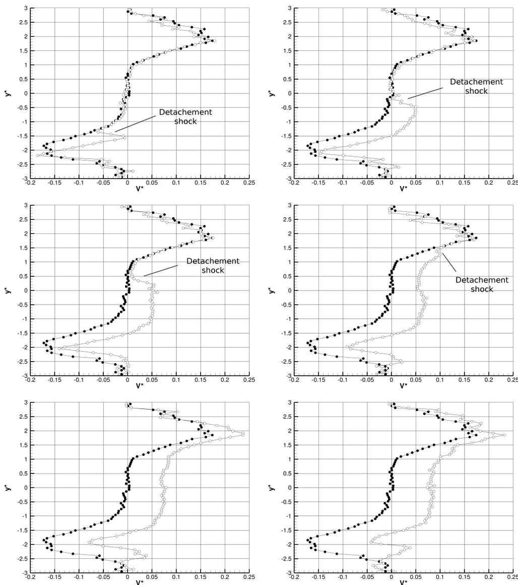
Figure 4: Vertical component of velocity  $V^*$  profiles at  $(x^*, z^*) = (0.4, 0)$ . ●: Unmanipulated case, ○: vectorized cases (from top to bottom and left to right :  $\Delta Q = 0.31\%$ ,  $\Delta Q = 0.63\%$ ,  $\Delta Q = 0.78\%$ ,  $\Delta Q = 1.0\%$ ,  $\Delta Q = 1.3\%$ ,  $\Delta Q = 1.62\%$ )
