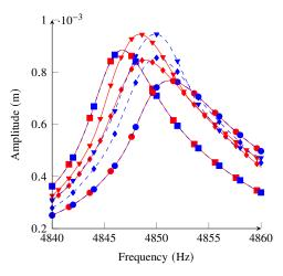
FIGURE 6: FREQUENCY FORCED RESPONSES FOR THE 1T MODE. (--): REFERENCE METHOD; (--): SNCR. THE MARKERS (II), (•), (•), AND ( $\forall$ ) DENOTE THE (A)<sub>24</sub>, (B)<sub>24</sub>, (AB)<sub>12</sub>, AND (ABBA)<sub>6</sub> STRUCTURES.
