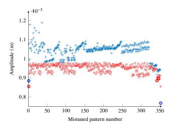
FIGURE 9: MAXIMAL AMPLITUDE DISPLACEMENT FOR THE DIFFERENT MISTUNING PATTERNS FOR THE 1T MODE. (**D**): COMBINATION OF AB AND BA; (+): COMBINATION OF AA AND BB.
