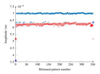
FIGURE 8: MAXIMAL AMPLITUDE DISPLACEMENT FOR THE DIFFERENT MISTUNING PATTERNS FOR THE 1F MODE. ([]): COMBINATION OF AB AND BA; (+): COMBINATION OF AA AND BB.
