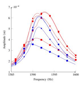
FIGURE 10: FREQUENCY FORCED RESPONSES FOR THE 1F MODE FOR THE SIX BEST STRUCTURES. (—): WITHOUT RAN-DOM MISTUNING; (—): WITH RANDOM MISTUNING. THE MARK-ERS (**m**), (**v**), (**o**), AND (**o**) DENOTE THE (A)<sub>24</sub>, (AB)<sub>12</sub>, (2A2B1A1B)<sub>4</sub> AND MP345 SYSTEMS.
