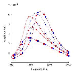
FIGURE 5: FREQUENCY FORCED RESPONSES FOR THE 1F MODE. (--): REFERENCE METHOD; (--): SNCR. THE MARK-ERS (II), (•), (•), AND ( $\forall$ ) DENOTE THE (A)<sub>24</sub>, (B)<sub>24</sub>, (AB)<sub>12</sub>, AND (ABBA)<sub>6</sub> STRUCTURES.
